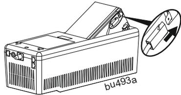
4 Reinstall the battery compartment cover. Be sure that the release tabs lock into place.
