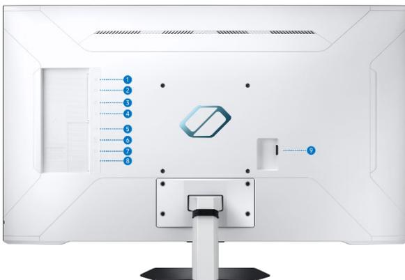
● USB ● USB (PC IN) ● USB ● Headphone IN ● DP IN ● HDMI IN ● HDMI IN ● LAN ● POWER
