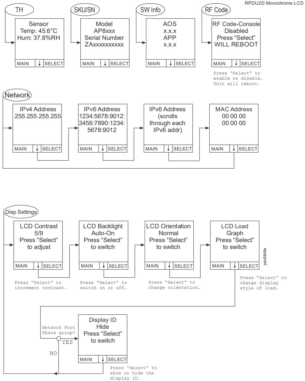
**NOTE:** RF Code is only available for Rack PDUs with NMC2s (firmware v6.x.x).
