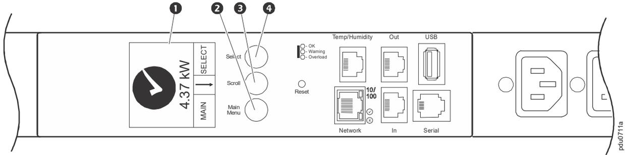
**NOTE:** Your Rack PDU is configured so the display backlight turns off after 10 minutes of inactivity. The backlight can be turned on by depressing any button below the display.
