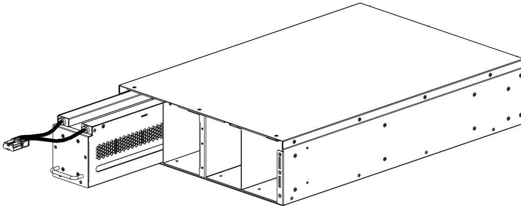
5 Mount the UPS and battery pack to the stabilizer bracket.
