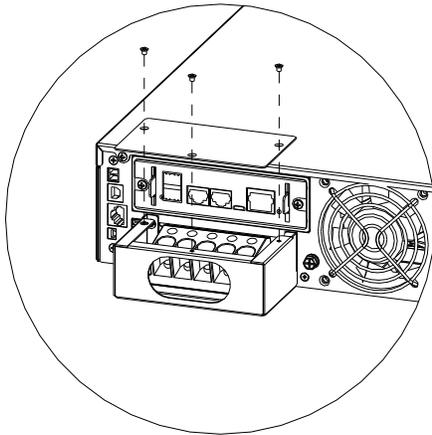
❷ Pass the input and output wires through the opening in the housing. The output ground wire is connected to the outer shell.
