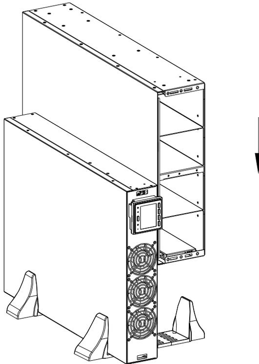
6 Rotate the LCD of UPS module 90 degrees to the right.
