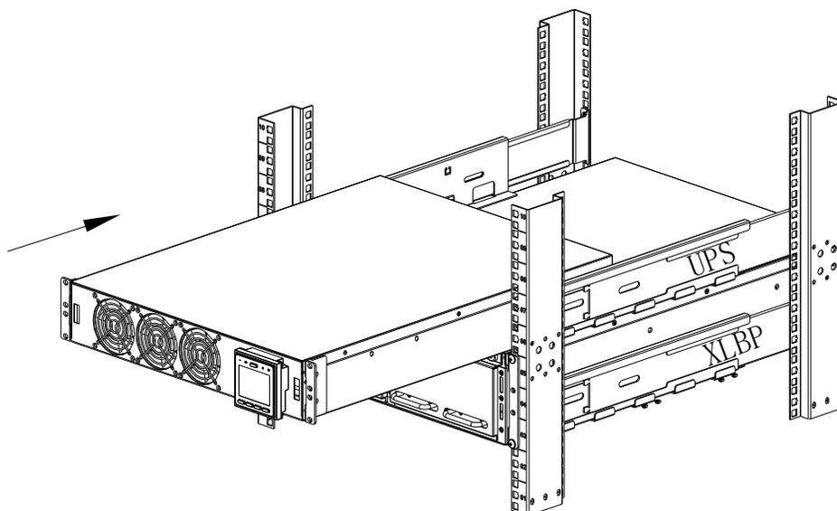
6 Secure brackets to pillar with 4 (M5x12) screws.
